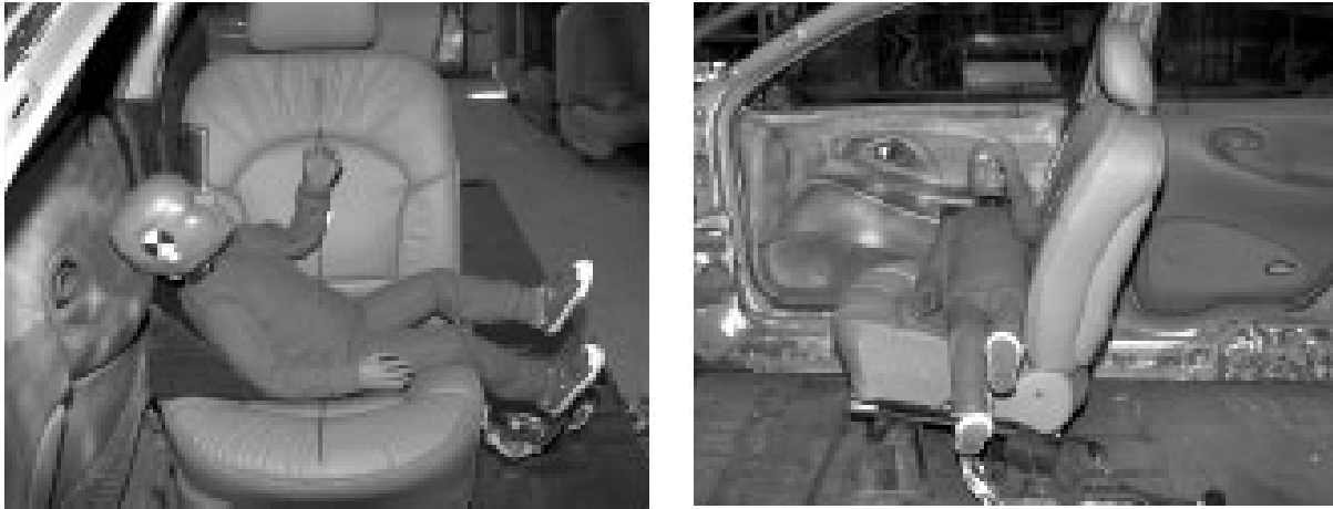
Figure 3.3.2.3.1 Hybrid III 3-Year-Old Child Dummy Lying Across Seat with Head on Door Trim Panel
