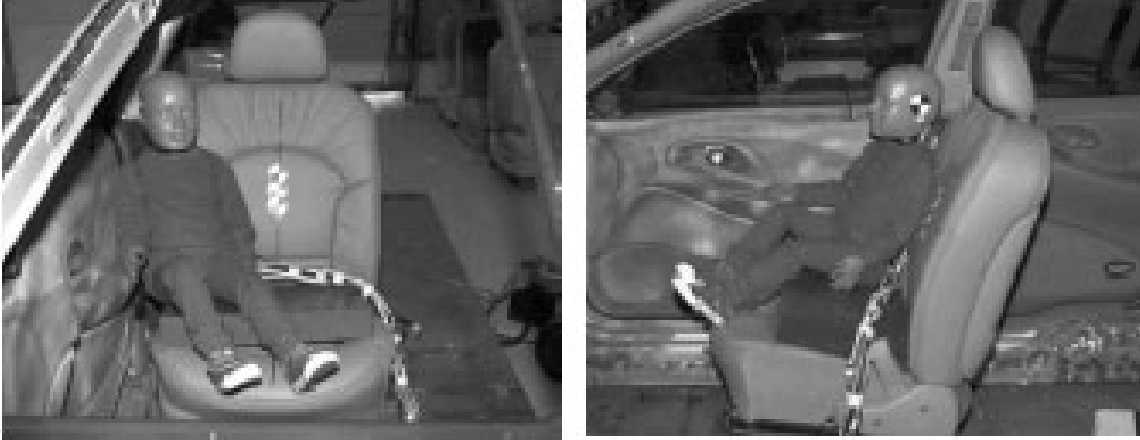
Figure 3.3.2.1.1 Forward Facing Hybrid III 3-year-old Child Dummy on Booster Block Leaning Against Door Trim Panel
